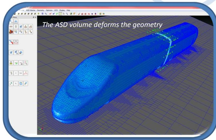
5 Control groups were defined with individual deformation vectors based on manufacturing constraints and realistic aerodynamic estimations. These groups were used as design variables in the setup of the optimization.
